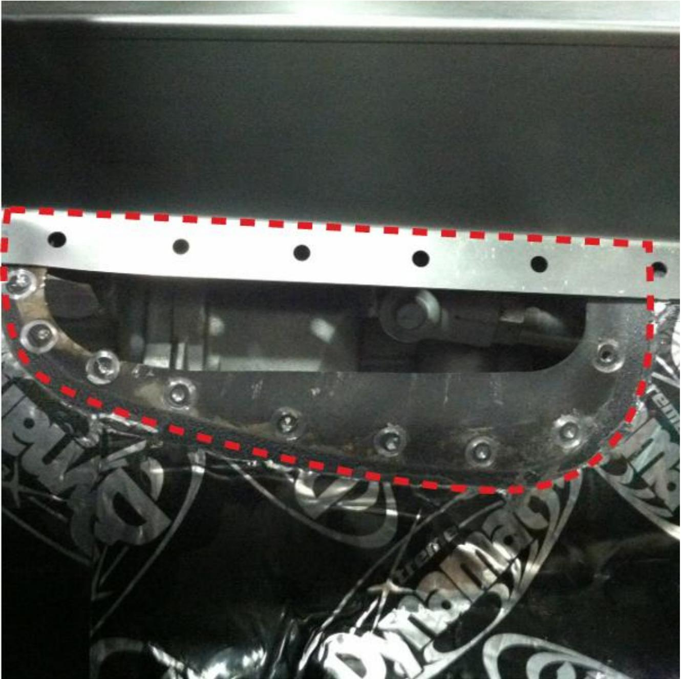
5. Some slight modification may be required to custom fit your tunnel cover to your specific car. Most common is bending the forward edge up to match the rise towards the firewall, and some slight trimming on the rear to match the contour of the tunnel, see illustrations below.
