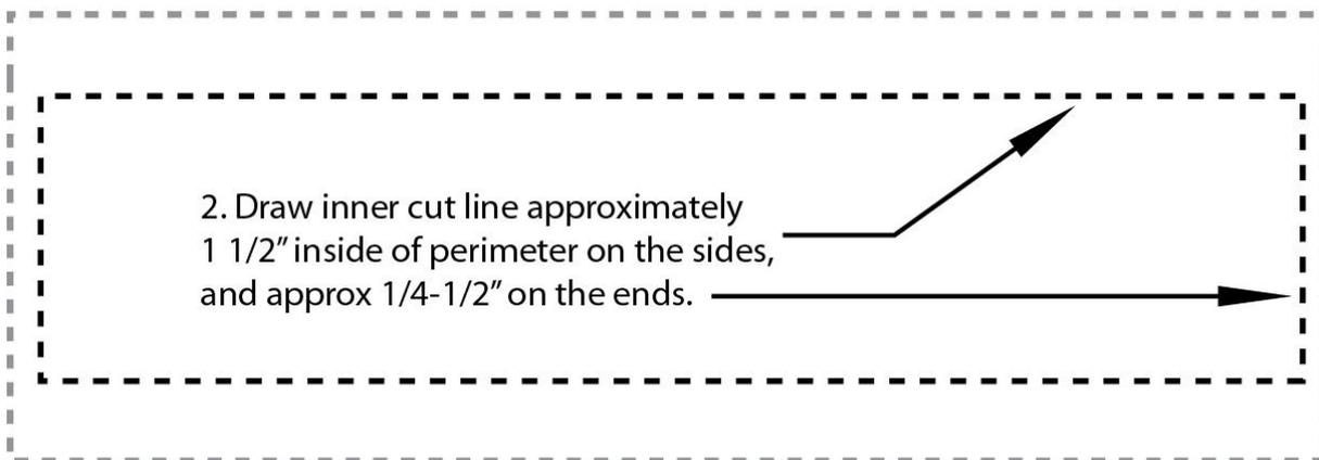
3. Once your cut lines are laid out, take the necessary safety precautions and carefully cut out the rectangular portion of the tunnel within your marks. Test fit the transmission in place. Because of model differences and factory tolerances further trimming may be required. Be sure there is a small amount of clearance to allow the drive train to flex without hitting the floor. The end result should look something like this
