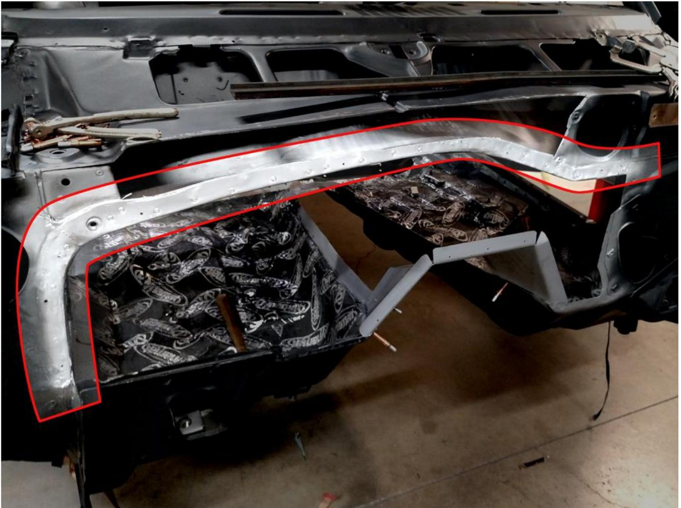
**4.** Proceed to cut along your marked cut lines and remove the old firewall. Mock up your new firewall in place. You can hold it with sheetmetal screws, clecos, etc.
