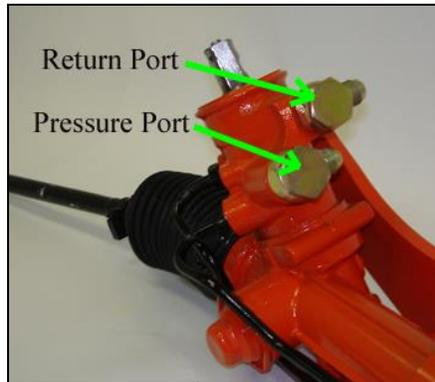
If you are using the new “GEN II” style pump please be sure to closely follow the accompanied pump installation instructions. Use **ONLY** power steering fluid in this pump and add the fluid to the pump slowly. The rack must be rotated slowly as you add the fluid.
