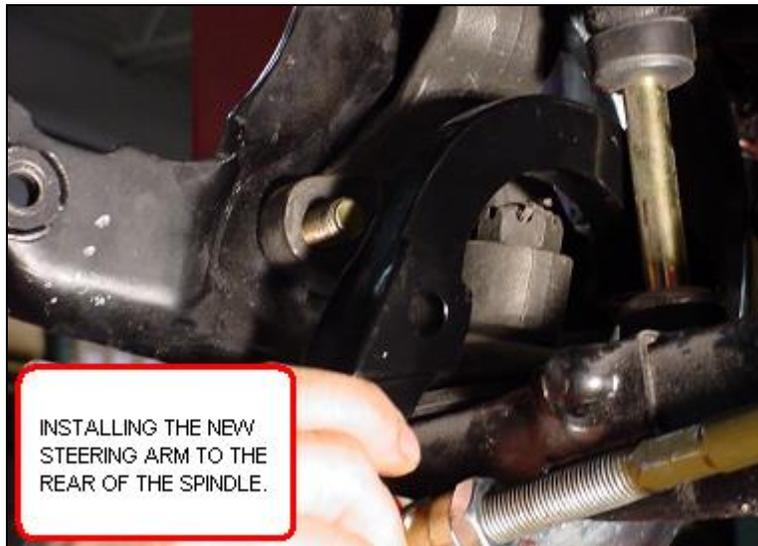
6) Adjust the outer tie rod ends so that each side is on equally (see next page). Insert the outer tie rod stud into the steering arm hole and nut the stud. Torque to **35 ft/lbs.**
