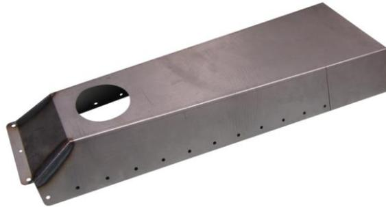
5. Now fit the remaining two portions of the cover on the floor. All three main parts get narrower as they go towards the back and can only be installed this way. Make a mark on the rear floor where the complete tunnel cover ends. Starting from there cut another 4" wide hole forward to the first area you removed. The end result will be a long hole front to back.
