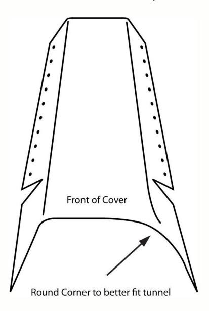
**3**. Once the tunnel cover is located properly and fits snug, mark and cut a hole approximately  $3\frac{3}{4}$ " (3.75) in diameter over where the shifter will be located. See also (**C**) on the next page. Fit and attach the pre bent cap on the rearward end (left side as pictured) of the cover as seen below.
