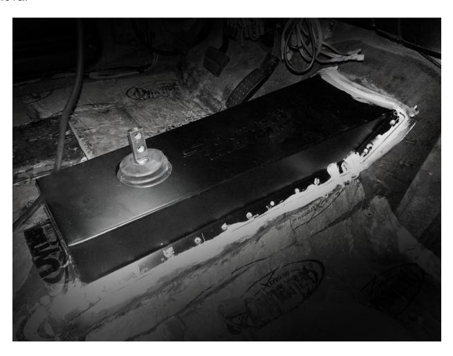
**7.** Cover your tunnel cover as fits your needs. We recommend splitting and securing vacuum tubing around the diameter of the shifter hole to prevent the metal edge gouging the transmission's rubber shifter boot. Because the cover design is fairly low it will easily accommodate a custom center console.
