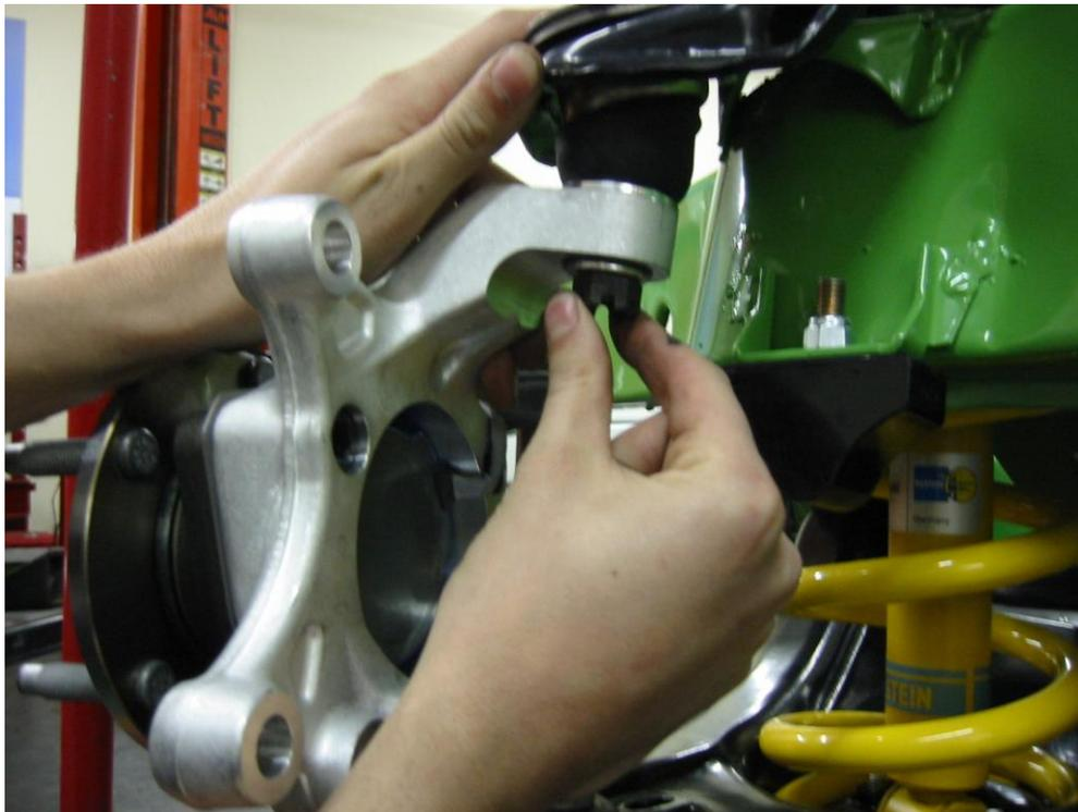
5. Make a careful note of shim placement and quantity used for the upper control arm alignment. Remove the two nuts holding the upper control arm shaft to the control arm mount and remove the upper control arm. Clean, remove rust and repaint the frame as needed.
