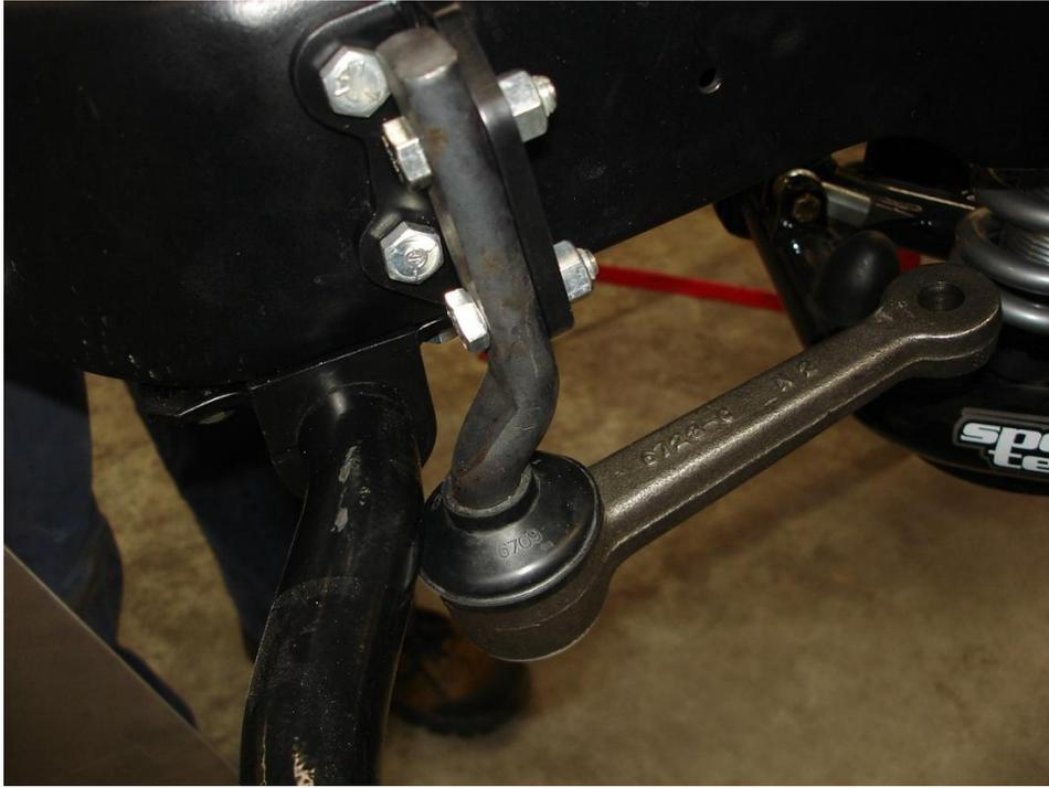
11. Assemble the inner tie rod ends, adjuster sleeves and outer tie rod ends.
