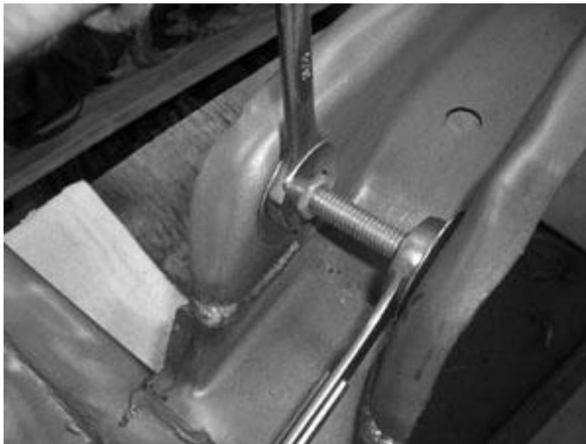
Spread the mount apart as needed by tightening the nuts against the frame.
