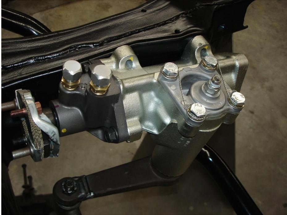
10. Install the idler arm relocation bracket on the frame and the idler arm on the bracket.
