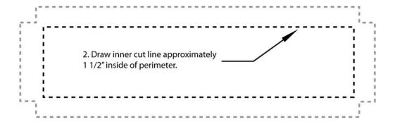
3. Once the cut lines are laid out, take the necessary safety precautions and carefully cut out the rectangular portion of the tunnel within your marks. Test fit the transmission in place. Because of model differences and factory tolerances further trimming may be required. Be sure there is a small amount of clearance to allow the drive train to flex without hitting the floor. The end result should look something like this
