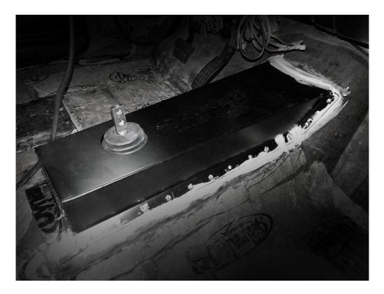
5. As the inside of the Tunnel Cover and the area of the floor pan covered by the Tunnel Cover may be exposed to outside elements, we recommend protecting these areas with a high quality paint or other surface protector. Attach the Tunnel Cover securely to the floor. We recommend using a high quality seam sealer on areas where the Tunnel Cover makes contact with the floor pan, and in any area where there may be flange gaps because of floor pan shape.
