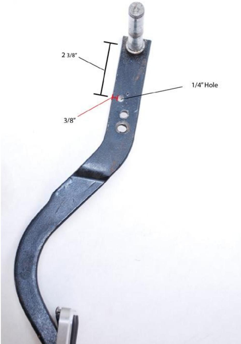
3. We recommend an adjustable clutch pedal stop be installed on the floor of the car to stop the pedal from bottoming out the clutch master cylinder. This is necessary to avoid bending the shaft. A simple 3/8" coupling nut bolted or welded to the floor will allow you to adjust a bump stop or bolt and jam nut to achieve the proper pedal travel.
