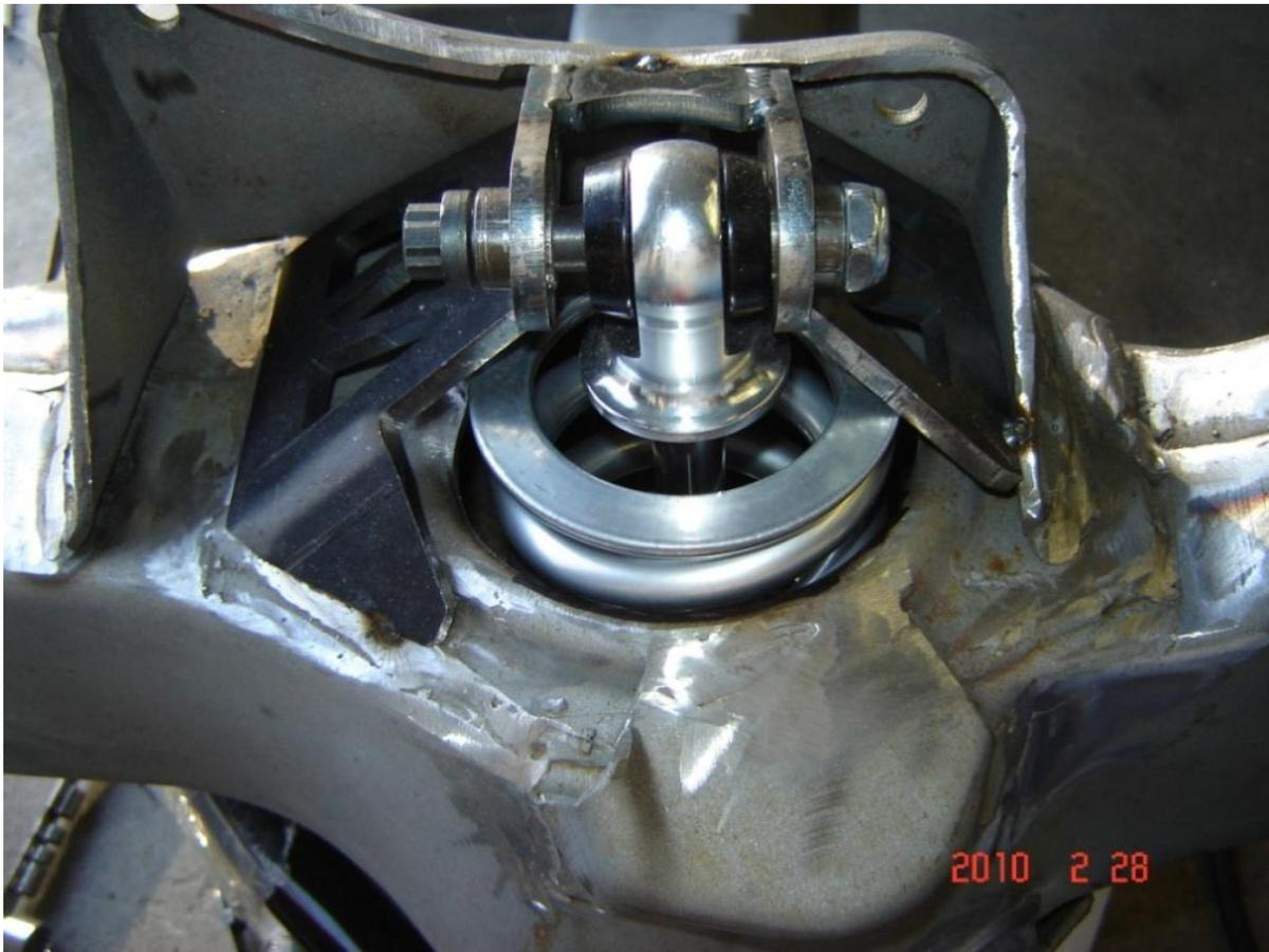
11. Remove the shock assembly and then remove the spring from the shock. Reinstall the shock into the lower control arm and the Chicane bracket to test again for any binding throughout the control arm's range of motion. Now that you have double checked everything and there is no bind and no clearance issues, you can final weld the Chicane upper bracket in place.
