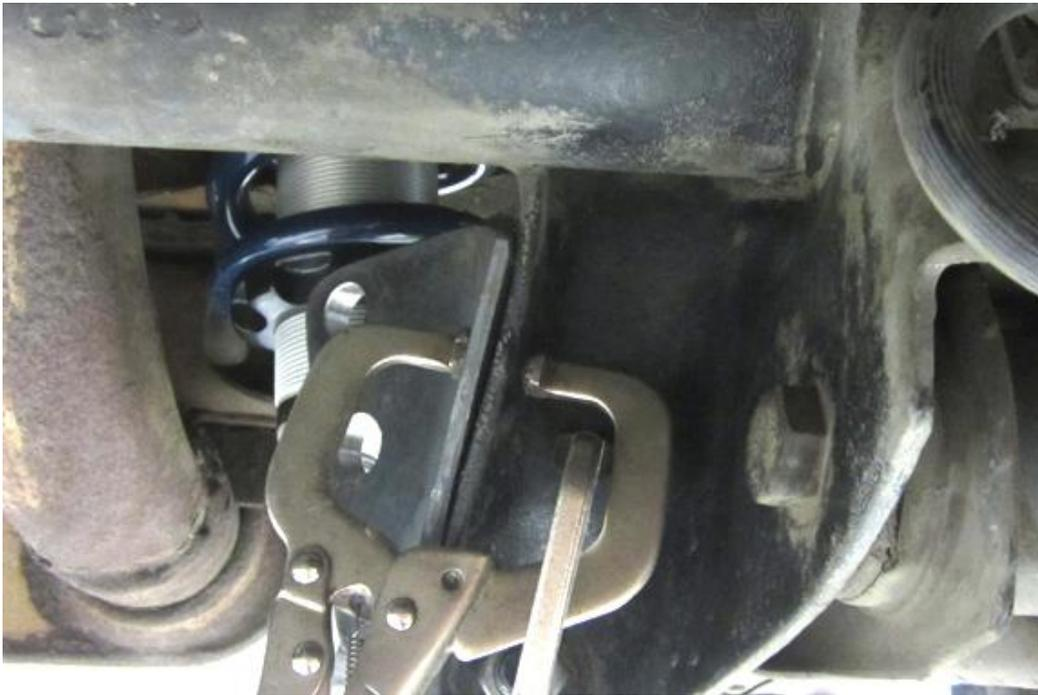
Measure and mark the rear side of the factory bracket 3" above the 1/2" bolt. Using your mark, drill a 7/16" hole through both the factory and Speedtech bracket. Install one 7/16 x 1 1/4", (2) 7/16" washers, and one 7/16" Nylock nut through the hole and tighten.
