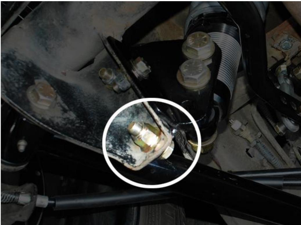
Next, clamp the bracket to the factory mount. This will keep it stable while you drill the two required holes.
