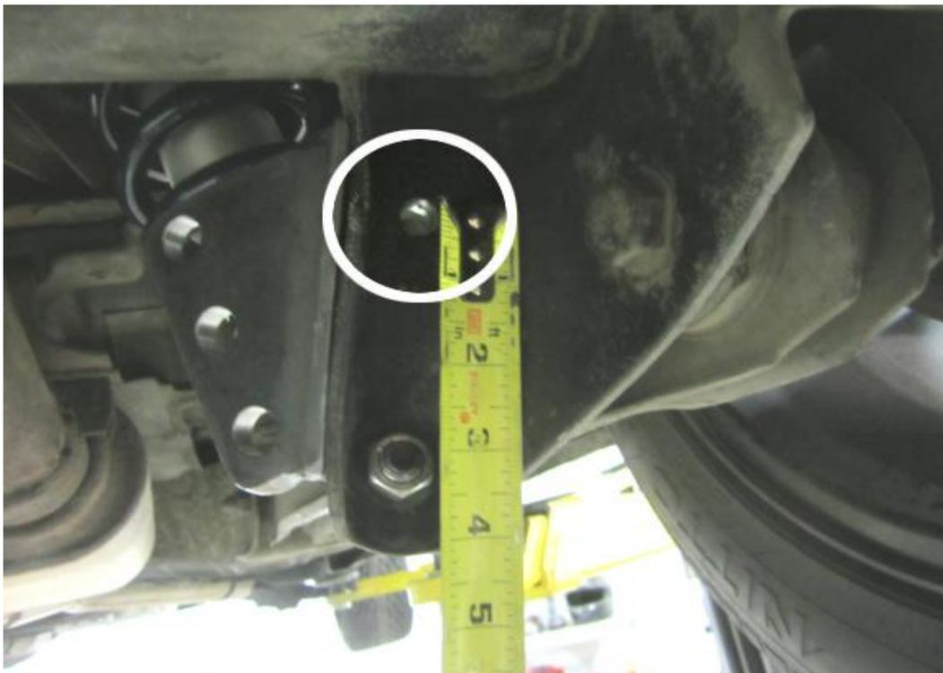
Using the pre-drilled hole in the Speedtech bracket as a guide, drill a 7/16" hole in the side of the factory bracket. Use one 7/16 x 1 1/4" bolt, (2) 7/16" washers, and one 7/16" Nylock Nut and tighten down.
