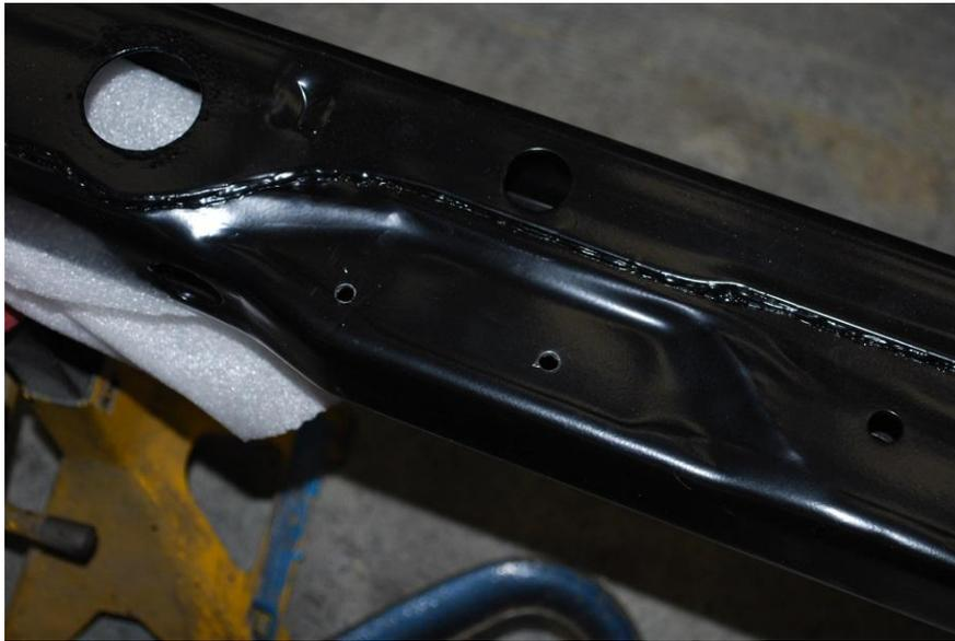
4. Now drill the **BOTTOM SIDE ONLY** with the 1" hole saw.
