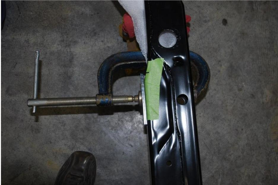
3. Using the  $\frac{1}{4}$  drill bit, drill up through the jig all the way through the frame rail.
