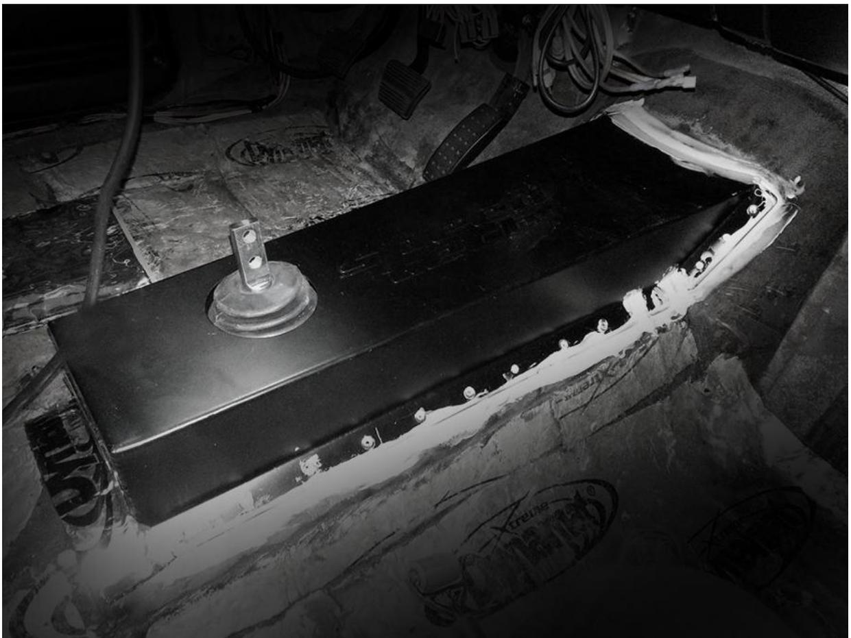
7. Cover your tunnel cover as fits your needs. We recommend splitting and securing vacuum tubing around the diameter of the shifter hole to prevent the metal edge gouging the transmission's rubber shifter boot. Because the cover design is fairly low it will easily accommodate a custom center console.
