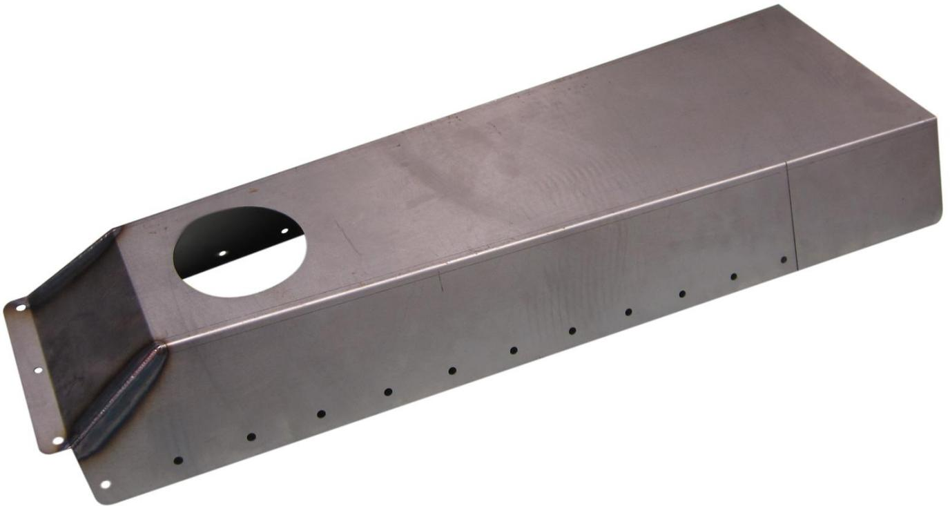
4. The front portion of the cover will need to be bent upward at the cut lines located on each side of the cover (**D**). This will help it better conform to the upward rise of the car's floor pan and bell housing area, see (**B**) below. Some hammer and dolly reshaping of the floor and tunnel cover will now be necessary for a closer fit to each other. With everything fitting well together trace a few of the pre drilled holes (**E**) onto the floor pan (**A**) for future alignment purposes.
